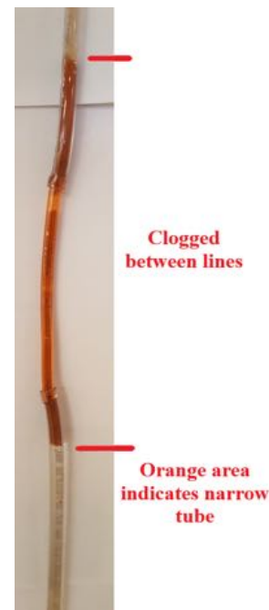
Figure 12. Sediment slurry forming a clog in extraction tubing during preliminary testing
