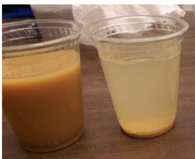
Figure 13. Gravity separation (left) vs electroflocculation assisted gravity separation (right)
